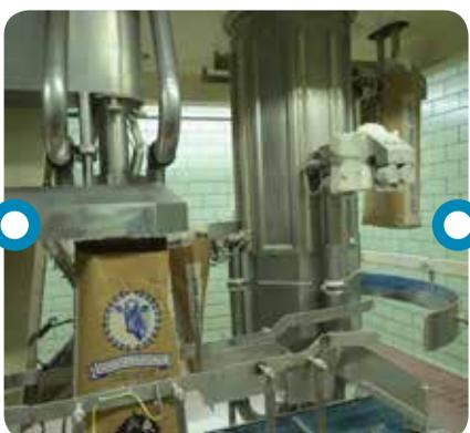
Powder is packaged by an automatic bagger.
