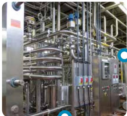
The plant utilizes a reverse osmosis system to remove water and produce skim condensed milk.
