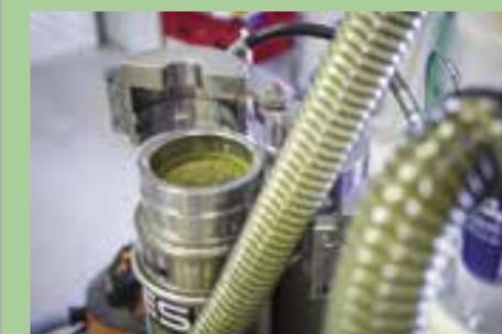
The hemp biomass goes through an extraction process at Ledge Rock Hemp to produce crude oil.
